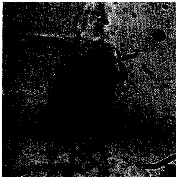
Figure 12. Photograph of catastrophic breakup of drop with a diameter of 69\ \mu\text{m} , under the action of an air jet velocity of 331\ \text{m/s} with a corresponding Weber number of 463.
