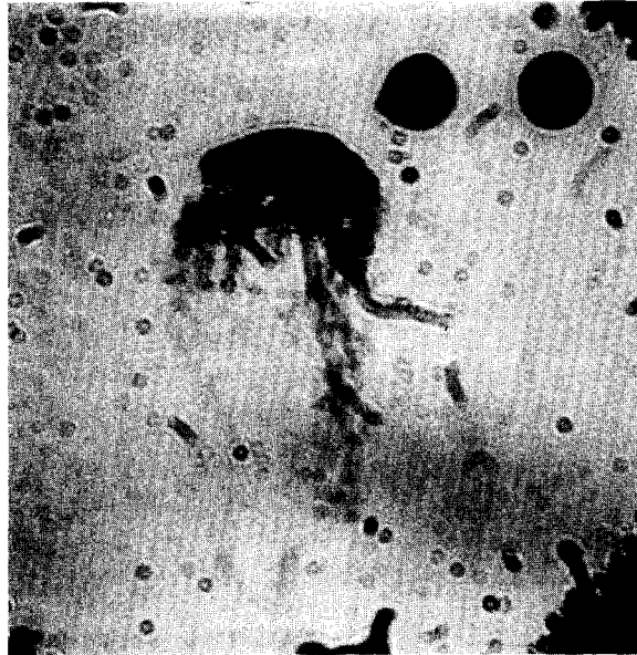
Figure 5. Photograph of shear breakup of drop with a diameter of 198\ \mu\text{m} , under the action of an air jet velocity of 147\ \text{m/s} with a corresponding Weber number of 260.
