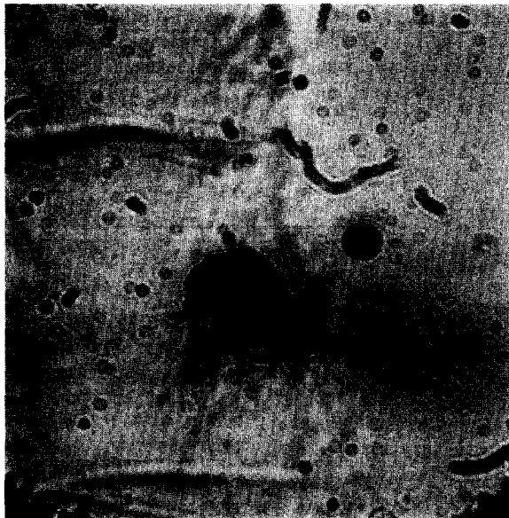
Figure 10. Photograph of shear breakup of drop with a diameter of 69\ \mu\text{m} , under the action of an air jet velocity of 248\ \text{m/s} with a corresponding Weber number of 260.
