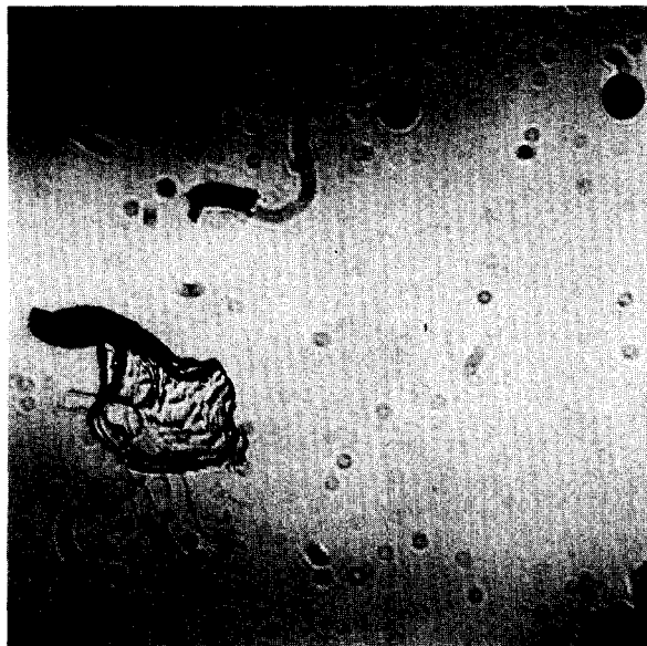
Figure 8. Photograph of bag breakup of drop with a diameter of 69\ \mu\text{m} , under the action of an air jet velocity of 115\ \text{m/s} with a corresponding Weber number of 56.
